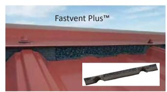
completely sealing against the panel profile. This form-fit reduces wind-driven rain problems to a minimum. Closed cell polyethylene completely surrounds the open-cell venting foam. Zero snow infiltration.
